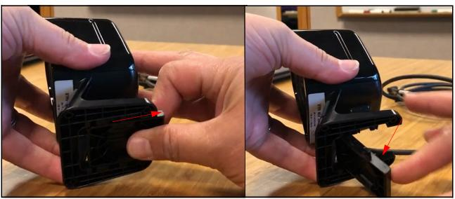
5. If installing the Riser, first open the Riser door to facilitate plugging in the cable. Pull the riser door straight out, then push down to swing open.
