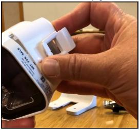
2. Affix the L Bracket to the desired surface using provided screws or similar. The head of the screw must not protrude above the main face of the bracket. Do NOT use flathead screws for installation.
