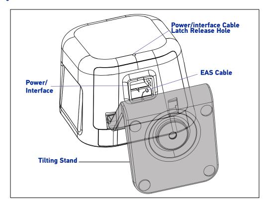
Figure 3. Scanner Features - Bottom View
