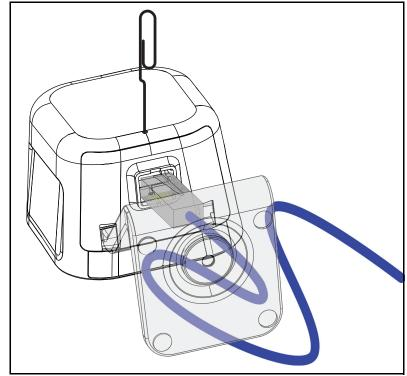
2. If the EAS cable is present, free it from the notch in the bottom cover before pulling the Stand away from the unit, as shown on page 7.
