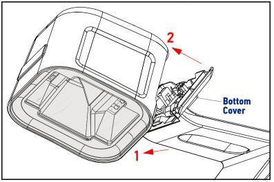
When installing the Riser, be sure to apply pressure only on the bottom cover, not the Riser foot.
